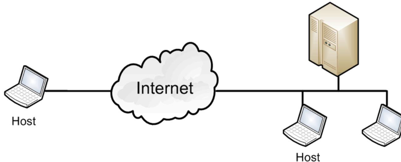
The least commonly used VPN architecture is the host-to-host model, which is typically used for special purpose needs, such as system administrators **performing remote management of a single server**.
