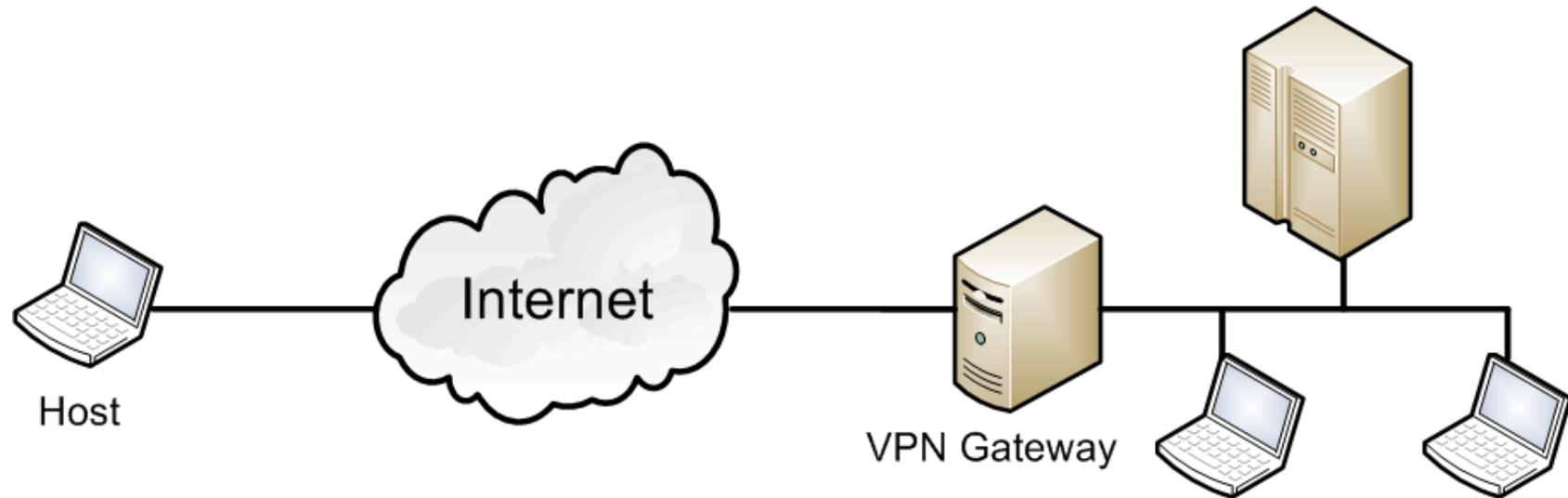
The client and gateway exchange information, and the IPsec connection is established. The user can now use the organization's computing resources, and the network traffic between the user's host and the VPN gateway will be protected by the IPsec connection.
