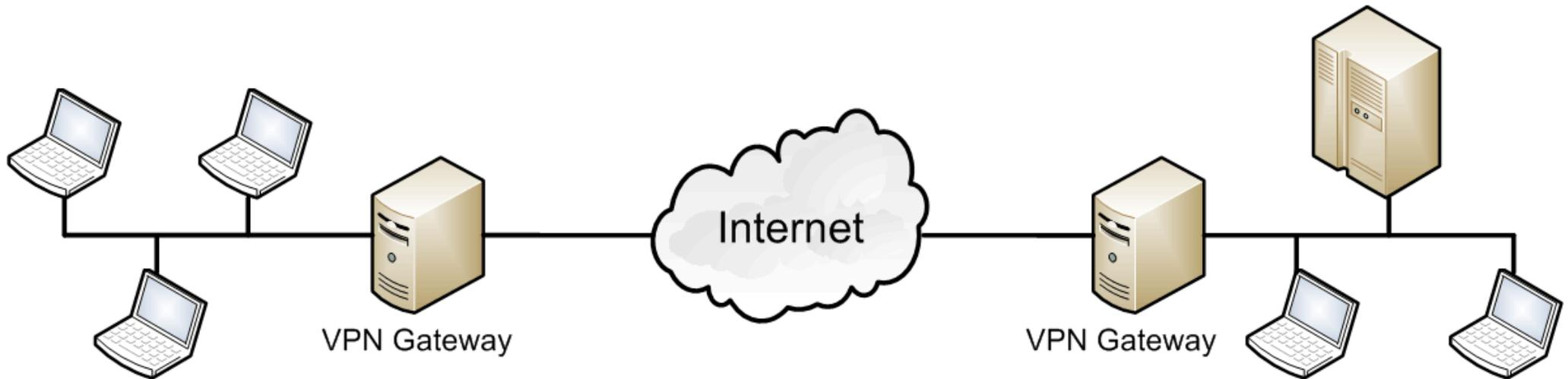
IPsec-based VPNs are often used to provide secure network communications between two networks. This is typically done by deploying a VPN gateway onto each network and establishing a VPN connection between the two gateways. Traffic between the two networks that needs to be secured passes within the established VPN connection between the two VPN gateways.
