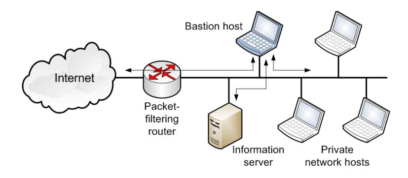
In **single-homed bastion configuration** the firewall consists of two systems: a packet-filtering router and a bastion host. Typically, the router is configured so that
