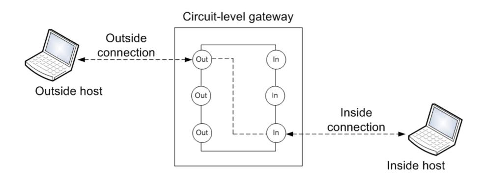
A typical use of circuit-level gateways is a situation in which the system administrator trusts the internal users. The gateway can be configured to support application-level or proxy service on inbound connections and circuit-level functions for outbound connections. In this configuration, the gateway can incur the processing overhead of examining incoming application data for forbidden functions but does not incur that overhead on outgoing data.
