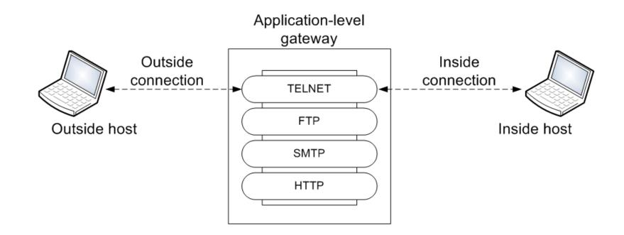
Application-level gateways tend to be more secure than packet filters. Rather than trying to deal with the numerous possible combinations that are to be allowed and forbidden at the TCP and IP level, the application-level gateway need only scrutinize a few allowable applications. In addition, it is easy to log and audit all incoming traffic at the application level.
