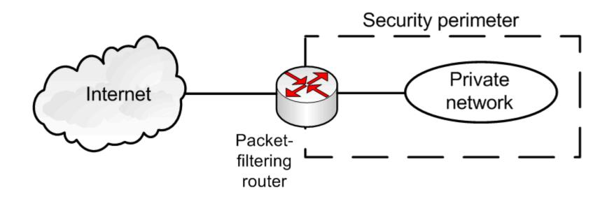
The packet filter is typically set up as a list of rules based on matches to fields in the IP or TCP header. If there is a match to one of the rules, that rule is invoked to determine whether to forward or discard the packet. If there is no match to any rule, then a default action is taken. Two default policies are possible:
