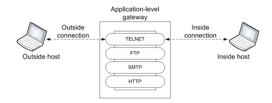
An application-level gateway, also called a **proxy server**, acts as a relay of application-level traffic. The user contacts the gateway using a TCP/IP application, such as Telnet or FTP, and the gateway asks the user for the name of the remote host to be accessed.
