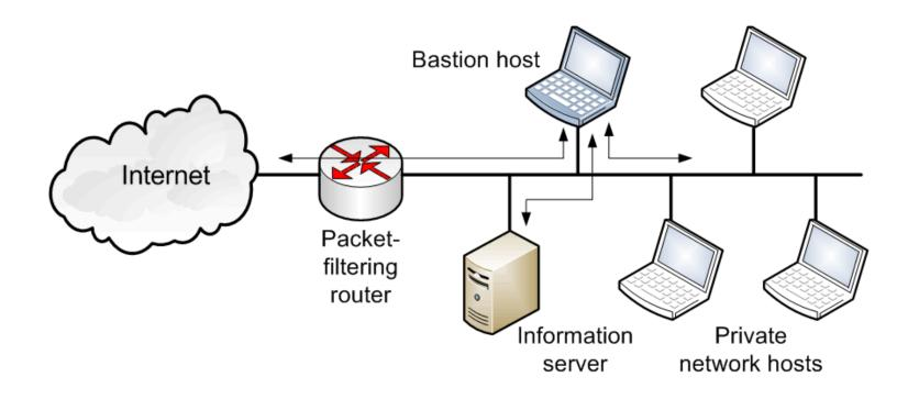
The bastion host performs authentication and proxy functions. This configuration has greater security than simply a packet-filtering router or an application-level gateway alone, for two reasons.
