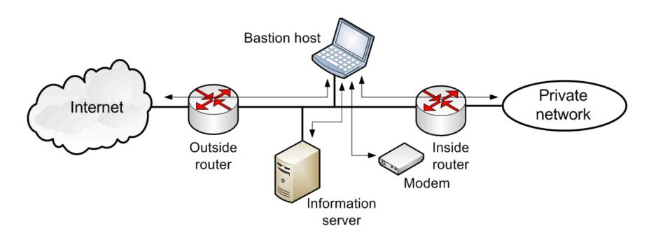
The **screened subnet firewall configuration** is the most secure of those we have considered. In this configuration, two packet-filtering routers are used, one between the bastion host and the Internet and one between the bastion host and the internal network. This configuration creates an isolated subnetwork, which may consist of simply the bastion host but may also include one or more information servers and modems for dial-in capability.
